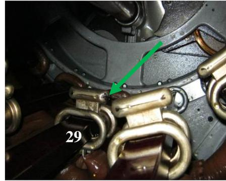
High current marks at contact 29, phase W
