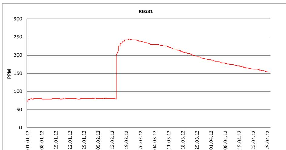
**Figure 11:** Gas content development during the period before and after the incident (Hydran)
