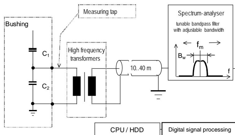
**Figure 6a:** Schema of measuring circuit for the PD measurement on a transformer bushing tap
