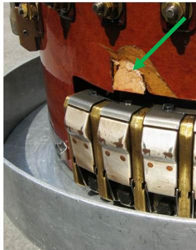
**Figure 13:** Mechanical damage on the OLTC-unit
