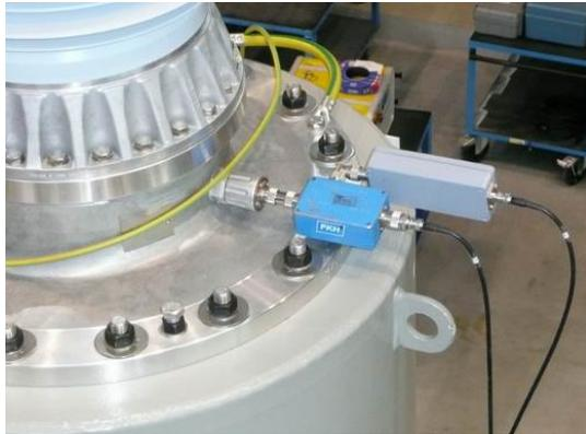
Installation of high frequency transformers and divider secondary capacitor on a bushing with measuring tap.
