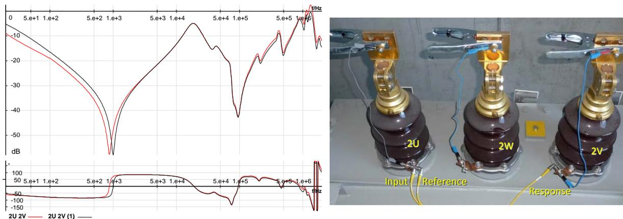
Example of the amplitude of the transferfunction as ratio of voltage (measurement from terminal 2Uu to 2V).
