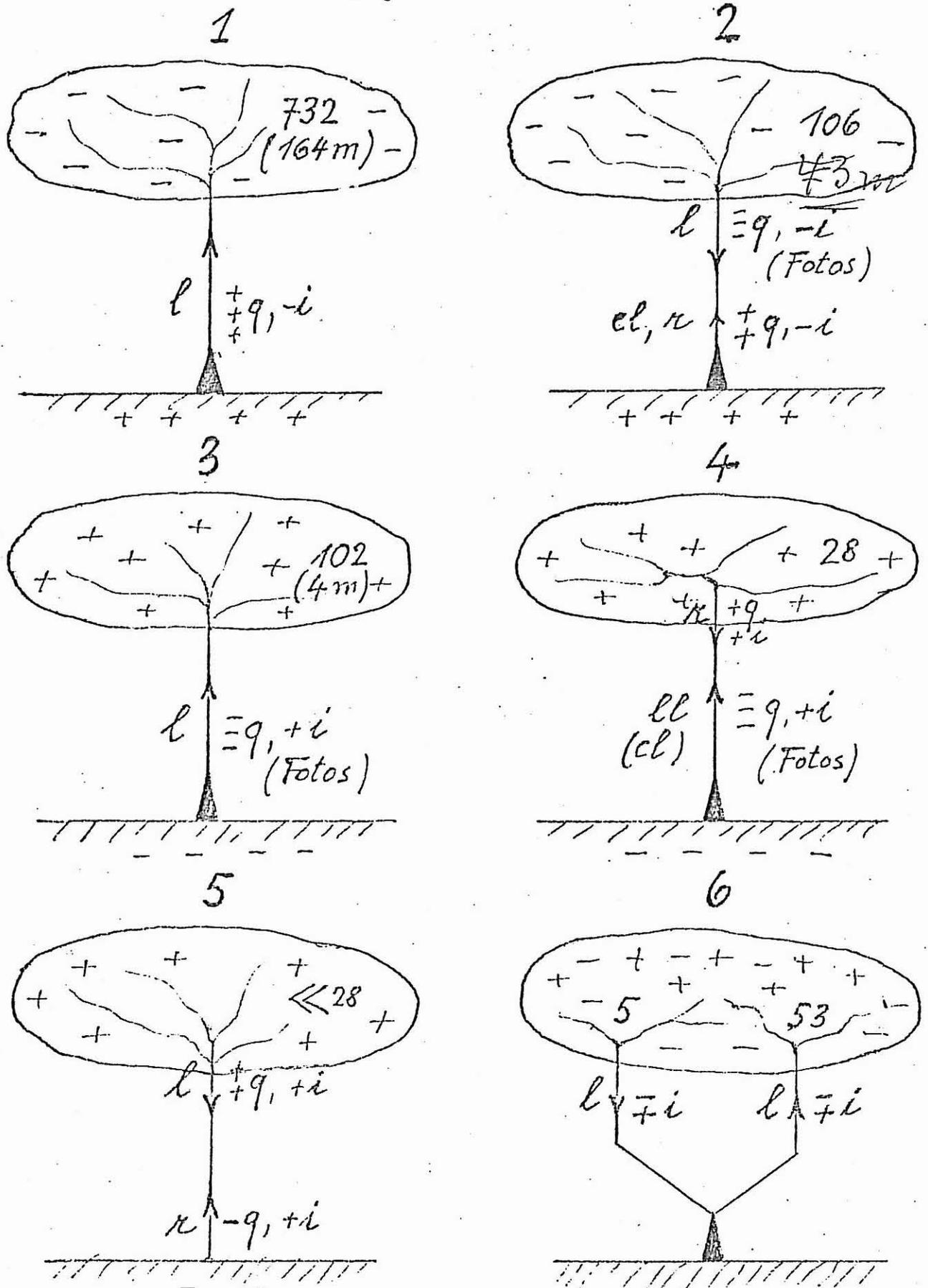
Fig. 1 Types 1...6 of lightning strokes to and from Mount San Salvatore
