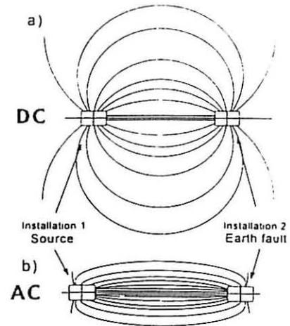
Figure 5 Lines of current in a resistive electric field between two earthing systems (qualitative representation) for both cases: AC top; DC bottom. An earth fault has been set up in installation 2, which is fed over a transmission line from installation 1. Note the concentration of current lines in the case of AC on the side of the line departure.
