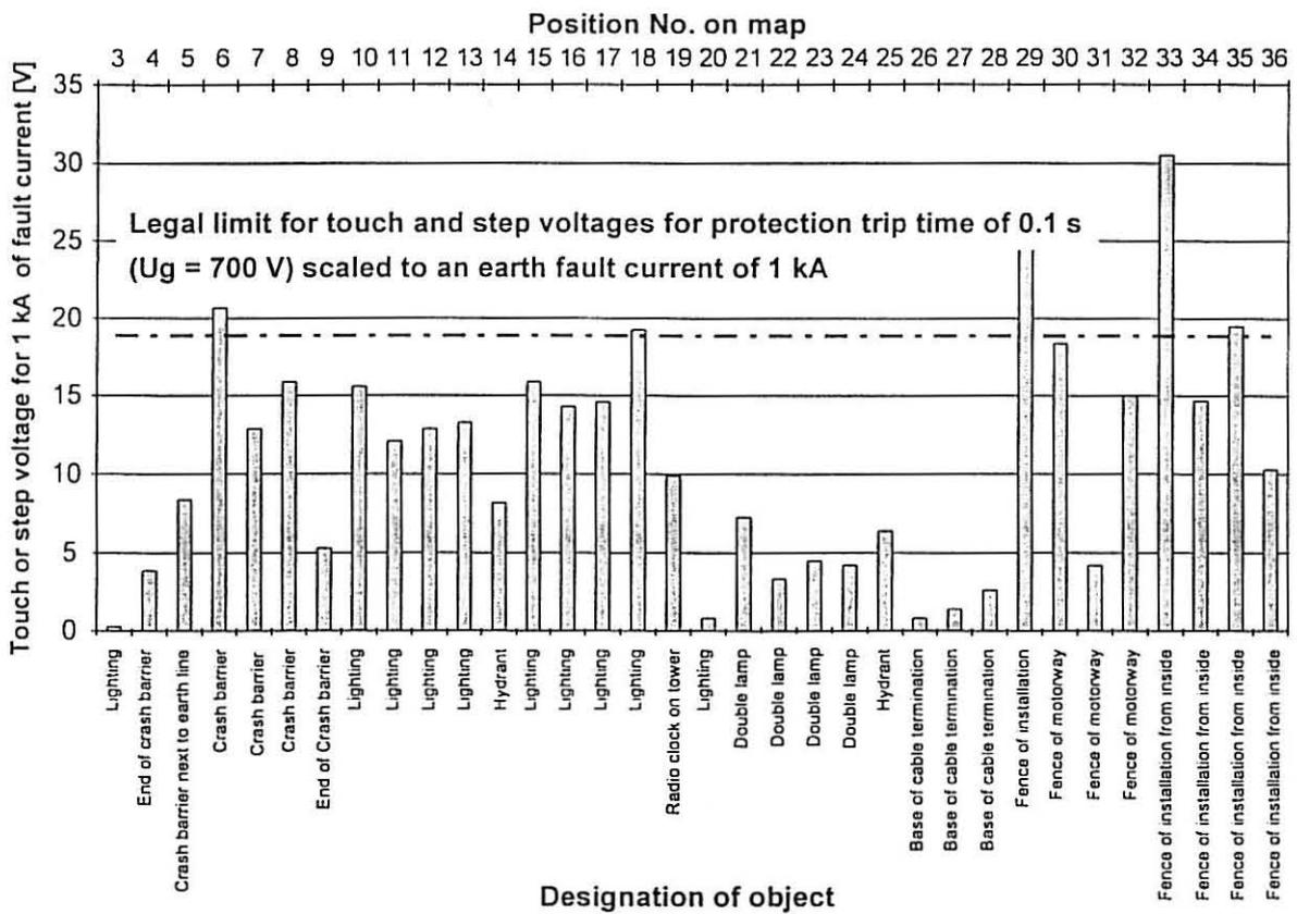
Figure 9 Graphic representation of measured touch and step voltages in the surroundings of a high voltage substation (for measured positions, see Figure 10).
