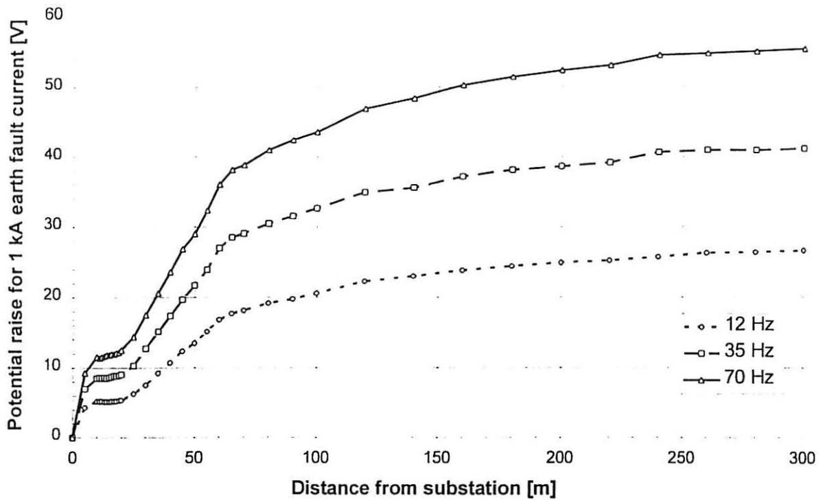
Figure 8 Voltage profiles of a 132 kV-substation measured at three different frequencies of the injecting fault current. The impedances to earth were estimated to 27 mΩ at 12 Hz, 41 mΩ at 35 Hz and 55 mΩ at 70 Hz.
