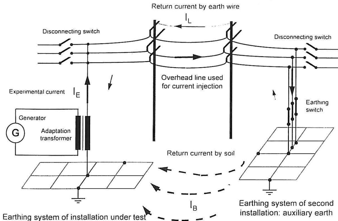
Figure 3 Formation of earth fault current loop by means of two substations and a connecting overhead line. The sum of the return current in the soil  $I_B$  and the return currents in the earth wire  $I_L$  results in the experimentally injected earth fault current  $I_E$ .
