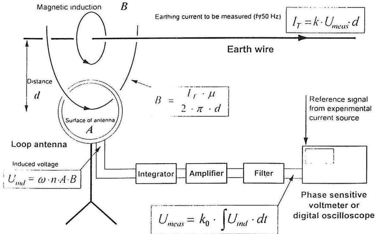
Figure 13 "Indirect" determination of earthing current shares in ground wires of overhead lines
