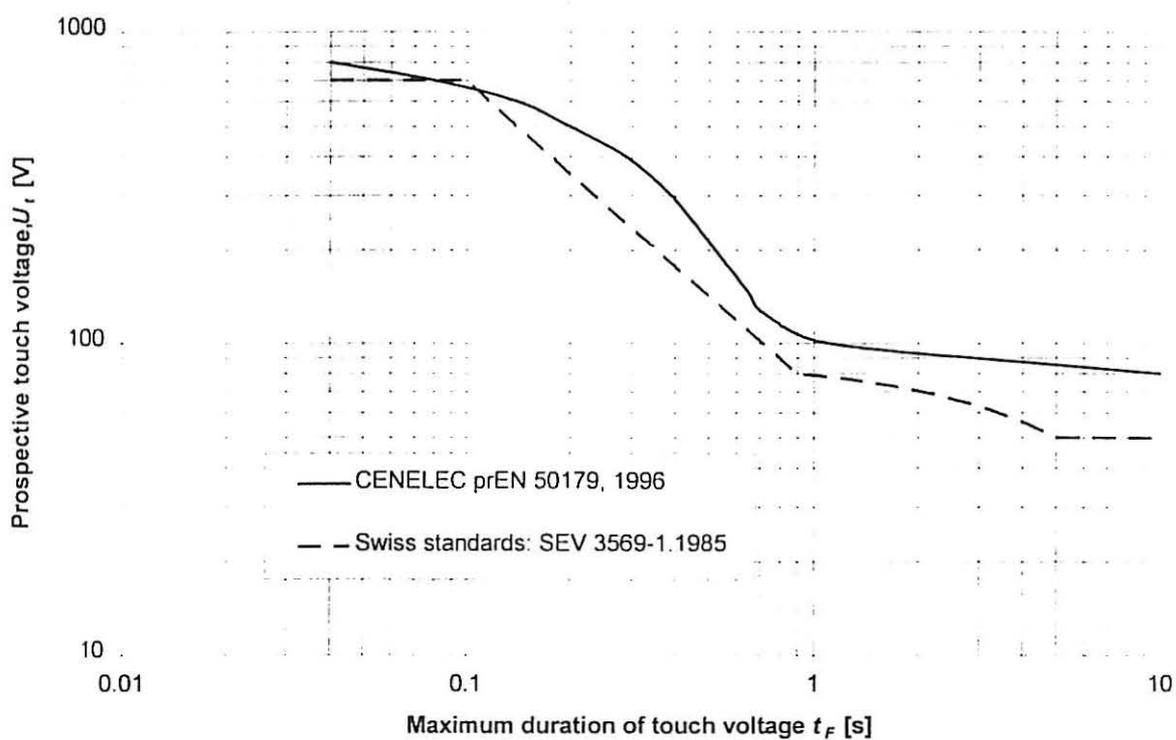
**Figure 1** Permissible touch voltages  $U_{Tp}$  for limited fault current flow duration.
