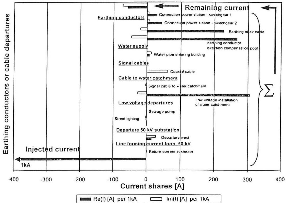
Figure 11 Example of a 'balance sheet'. Vectorial summation is required because of substantial phase shifts between the different shares of the earthing current.
