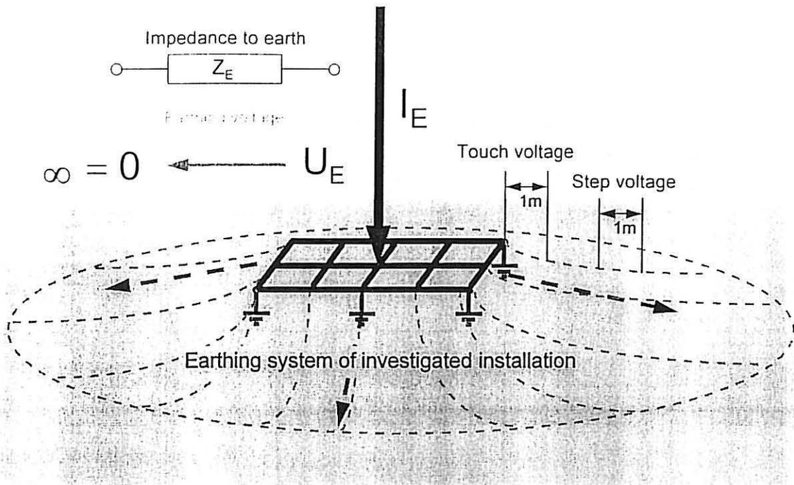
Figure 2 General principle of earthing measurements. An earthing fault current  $I_E$  is injected into the earthing system. This current flows through the soil and causes a potential rise  $U_E$  in the vicinity of the earthing system. Touch and step voltages are generated in the 'hot zone' around the installation.
