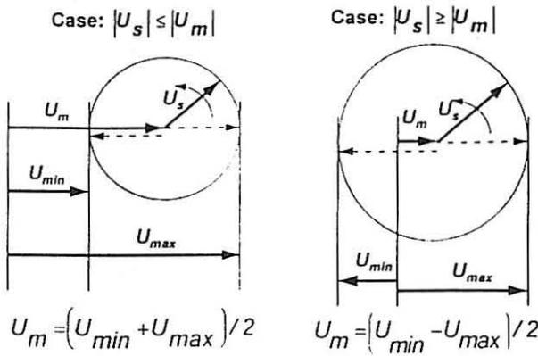
Figure 6 Determination of the measuring voltage with the beat method. The measuring voltage  $U_m$  is determined by eliminating the interference with mains frequency for the case that the measuring voltage is larger than the interference (left), and for the case that the measuring voltage is smaller than the interference (right).
