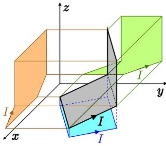
Figure 1. Projection of a non-complanate loop on three orthogonal planes
