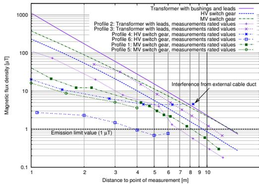
Figure 8. Theoretically evaluated and measured magnetic flux decay
