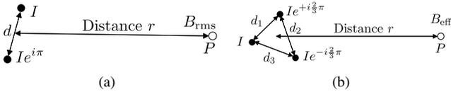
Figure 2. Definition of variables for the expression for the dipole magnetic flux density of (a) a two conductor line (eq. (5)) (b) a three-phase line (eq. (5) and (6))
