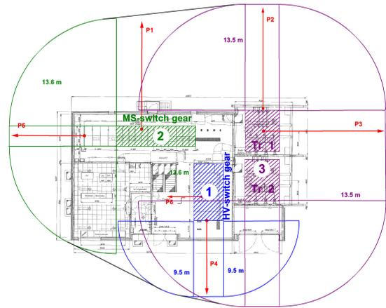
Figure 6. Result of a magnetic stray flux evaluation in a substation. The sum of maximum possible magnetic dipole moments for HV and MV switchgear and the transformers have been evaluated. The radius for the flux density to meet the emission limit of  $1 \mu\text{T}$  is plotted around the active installations
