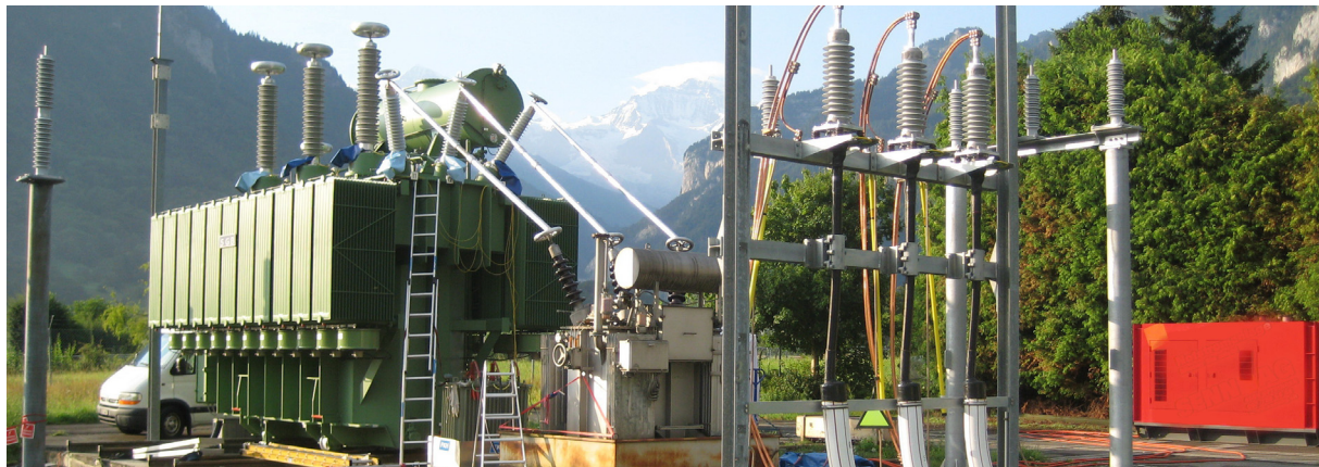
Figure 1: Example of an on-site test of a 75 MVA transformer (132/50 kV). In the middle the exciter transformer (0.4/50 kV); on the right side (red box) the diesel generator (360 kVA).
