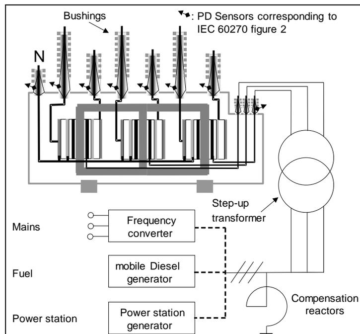
**Figure 4:** Example of different external voltage sources for on-site PD-measurements
