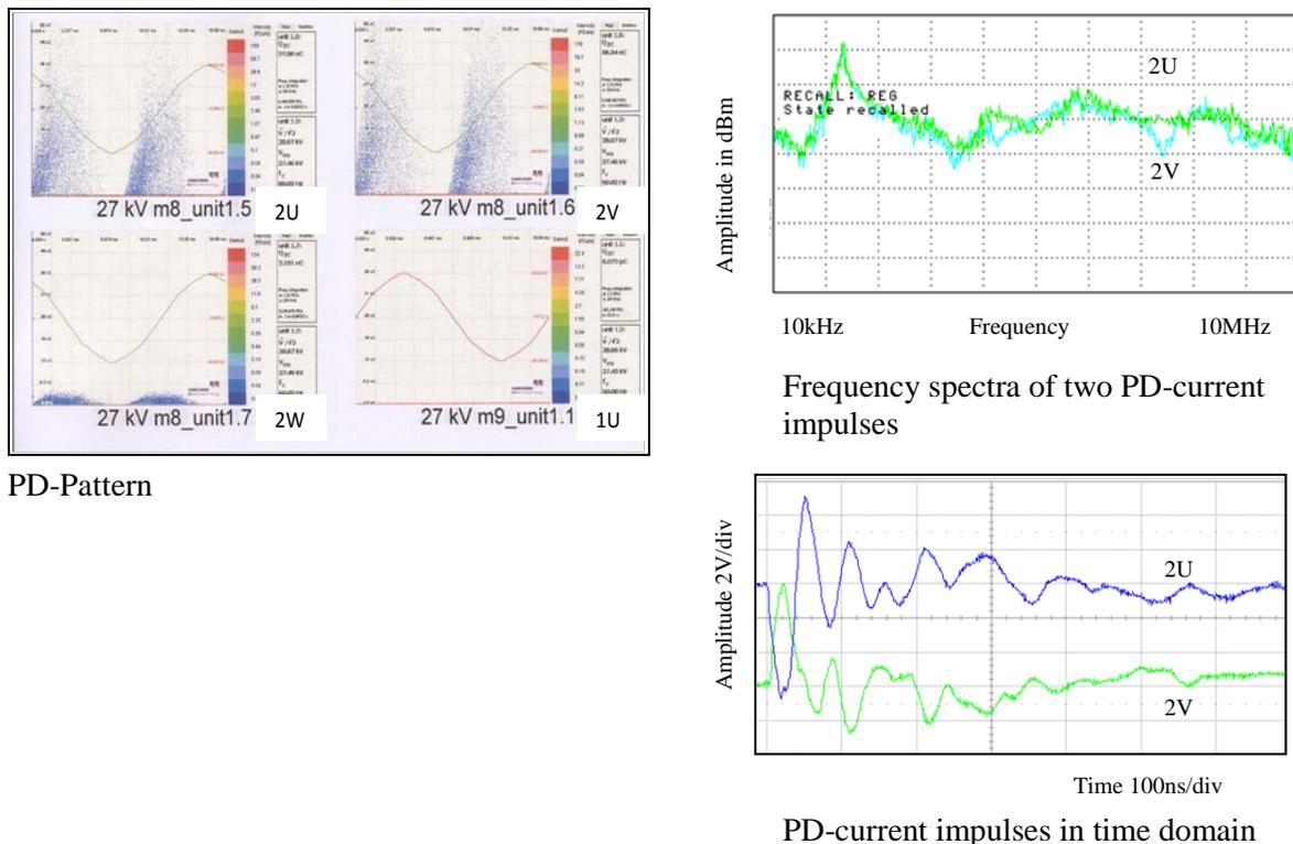
**Figure 7:** Typical results of PD-measurements
