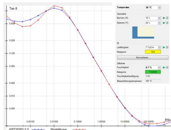
Measured and simulated loss factor  $\tan \delta$  in function of the applied voltage
