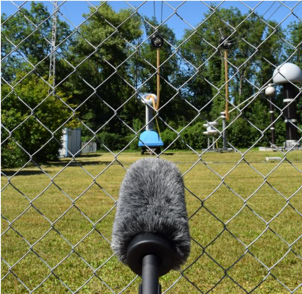
**Figure 4** Noise measurement with super-cardioid microphone
