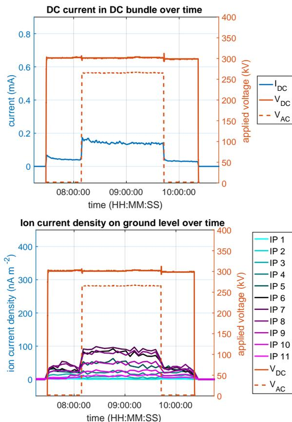
**Figure 6** Ground level DC ion currents (left) and DC corona current (right) under DC and hybrid operation
