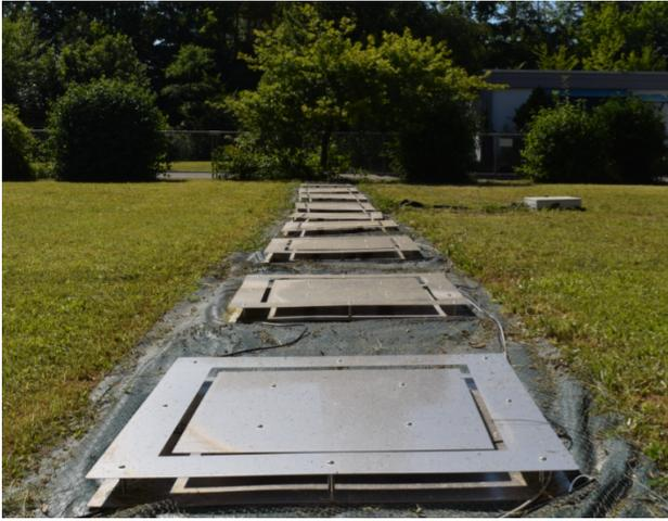
**Figure 2** Weatherproof Wilson ion current plates
