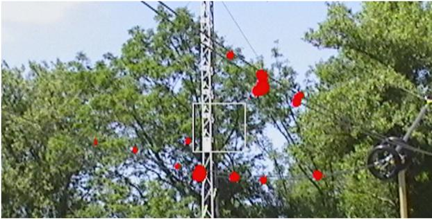
**Figure 5** Visual corona inspection using the UViRCO Corocam 7
