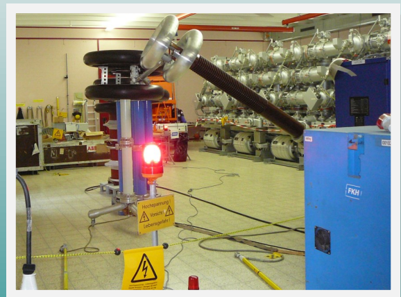
Voltage test with UHF partial discharge measurement on a 123 kV GIS S
