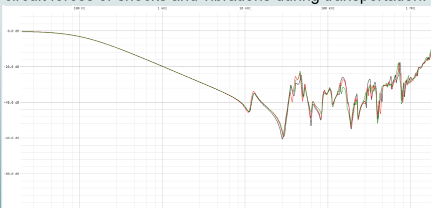
FRA measurements on a 3-phase transformer
