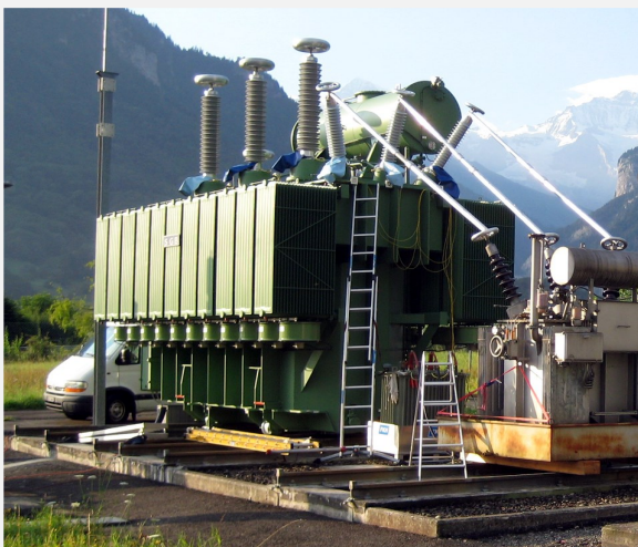
Excitation of a grid interconnection transformer for the partial discharge measurement in a substation
