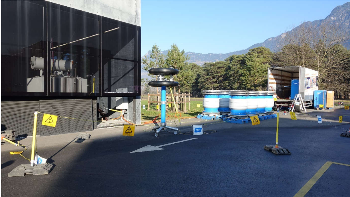
Figure 1: Barricading the test installation with warning flag cords
