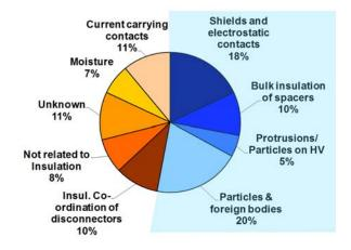
Figure 9: Main distribution of dielectric failures in service [12].
