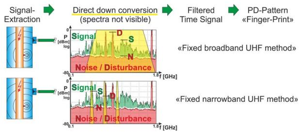
Figure 3: Illustration of fixed band UHF-PD measurement methods (spectra shown for illustration only, not actually measured by PDMS).
