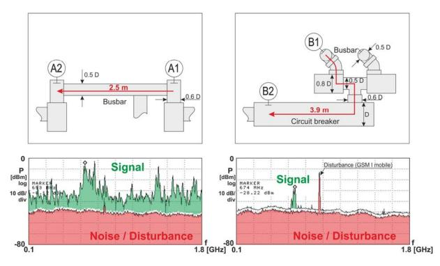
Figure 8: Bandpass characteristic with significant signal attenuation of a 3.9 m long 145-kV GIS section (single phase encapsulated).
