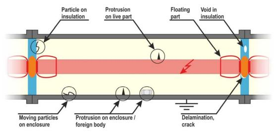
Figure 1: Typical fault types found in GIS installations.
