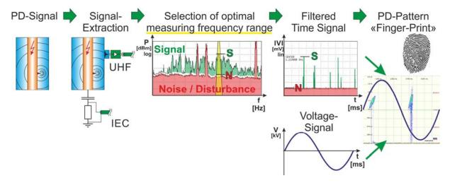
Figure 2: Classic narrow band UHF-PD measurement – illustration of signal processing.
