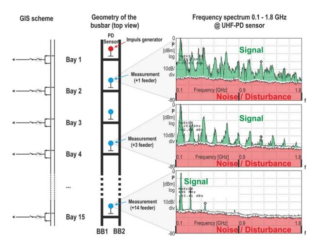
Figure 7: 245-kV GIS: Spectral signal attenuation along the double-busbar (50-dB preamplifier).
