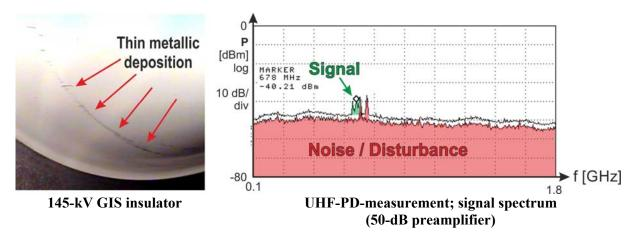
Figure 6: 145-kV GIS insulator with thin metallic deposit on its surface (distance between insulator and defect 2.5 m).
