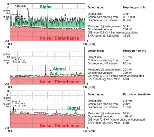
Figure 4: Spectral content of 3 different fault types measured on site; resolution bandwidth 3 MHz; critical defect sizes referenced in [10]; 50-dB preamplifier.
