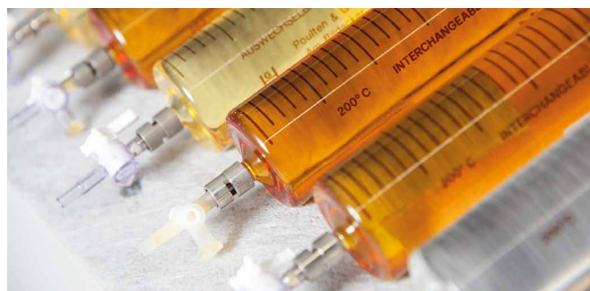
Figure 3: Oil samples for the analysis of decomposition gases
