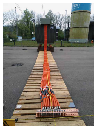
Figure 29: Magnetic field measurement on a 3.15 MVA distribution transformer
