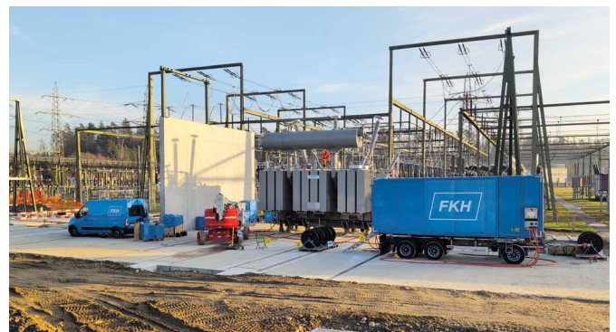
Figure 16: Partial discharge measurement using a mobile measurement unit (in a van) and a test trailer
