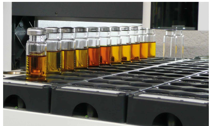
Figure 19: Vials containing oil for the analysis of dissolved gases in GC
