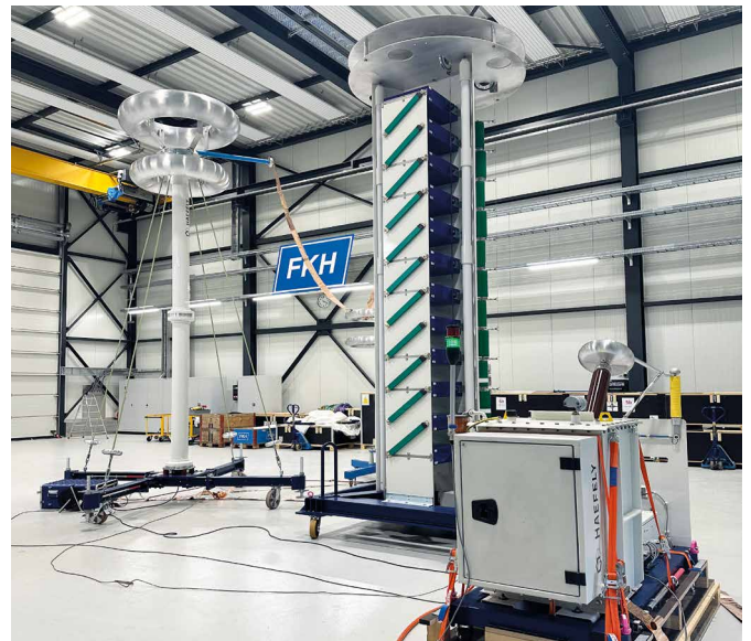
Figure 25: Modular pulse generator (shown here with 12 stages). In the foreground is the charging unit; to the left is the 1600 kV voltage divider
