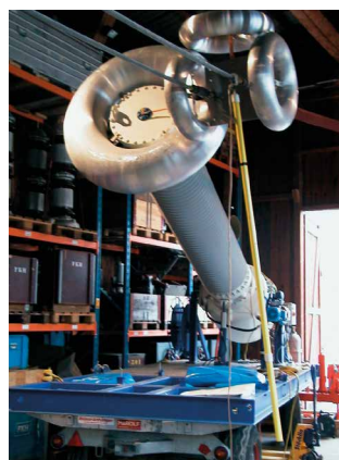
Figure 28: The gas-insulated 400 kV test transformer manufactured by Trench GmbH
