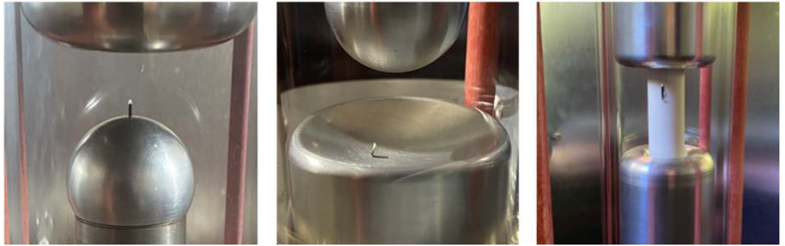
c) Needle on LV-potential - d) Free-moving particle - e) Particle adhering to insulator
