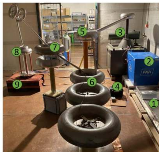
b) Experimental setup for UHF- and charge-based PD-measurements
